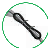
SPACE BELT CLAMPS LESS THAN 5" OR A FIST WIDTH APART
